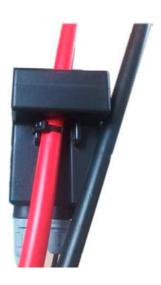
• In case of nominal currents corresponding to less than (or equal to) 100 A, fix the cable of the positive pole (red cable) twice through the hole of the SmartUP module, then fix it with the fairlead at the side of the module.
