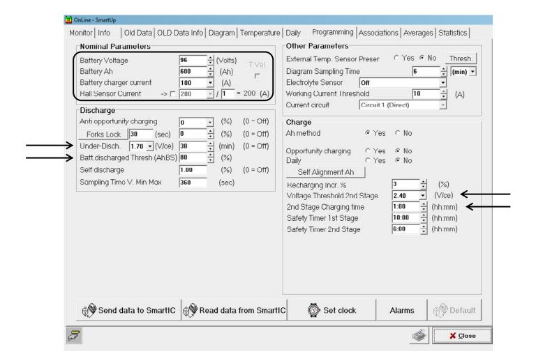
First of all configure the "Nominal parameters" selecting Battery Voltage (Volts), Battery Ah (capacity), Battery Charger Current (A), then set the Hall Sensor Current (A) depending on how the device is connected: the highlighted value in the figures below represents how many times the cable of the positive pole (red cable) passes through the Hall Sensor.
